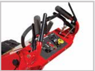
Need to walk away from the mower to move an obstacle or debris? The new PTO switch allows the operator to stop the mower blades in a single step – simply put the machine in neutral and release the controls. The blades will disengage while the engine continues to run.
