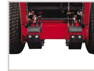
Foot pedal for neutral position provides the operator with more natural control. The neutral position is identified on the speed indicator on the dash.
