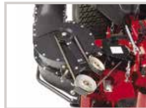
TURBO-Pro Max Blower — Length: 36" Height: 18" Width: 21" Approximate blower weight: 72 lbs. (52") / 64 lbs. (61"), includes mounting bracket
