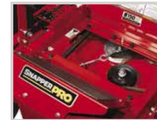
Quick removal of the floor pan provides convenient access to the top of the deck for easy cleaning and service.
