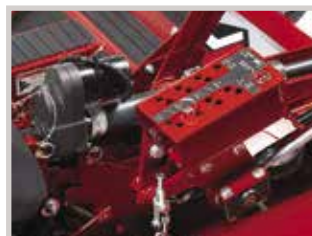
Electric deck lift makes for easy cut-height adjustment.
