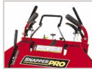
Reliably set your speed with the improved easy-to-reach cruise control bar featuring a speed indicator. Conveniently located brake handle.
